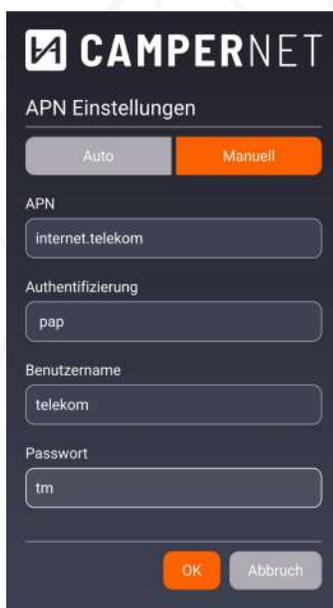
The screenshot shows the 'CAMPERNET' app interface for 'APN Einstellungen'. The 'Manuell' option is selected. The fields are filled with: APN: internet.telekom, Authentifizierung: pap, Benutzername: telekom, and Passwort: tm. There are 'OK' and 'Abbruch' buttons at the bottom.
